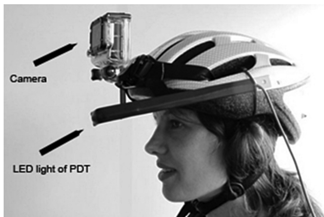
Fig. 2. LED light of PDT and camera for forward view.
