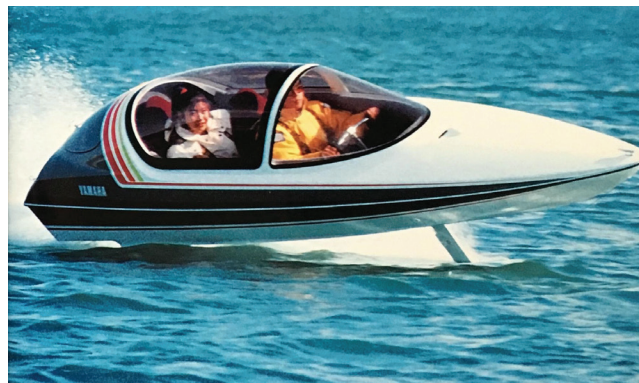
FIGURE 1. Kotaro Horiuchi has been designing and building single-track hydrofoil boats since the 1960's. Shown here is the OU32 single-track hydrofoil boat from 1988. [2]
