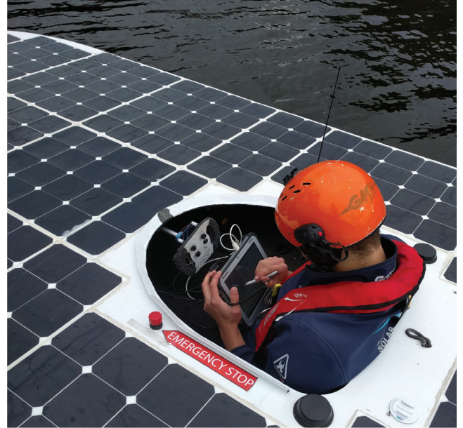
FIGURE 15. During tests, the crew is able to change the data-acquisition and height control software to find optimum settings. Data can be tracked live via a server and imported to software.
