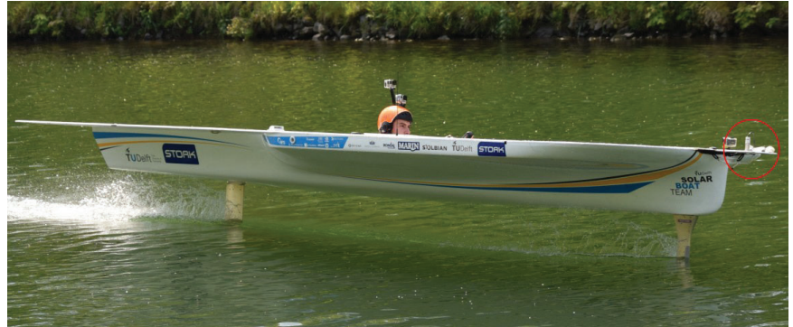
FIGURE 13. The Senix ToughSonic REMOTE 14 [12] constantly measures the height of the boat.
