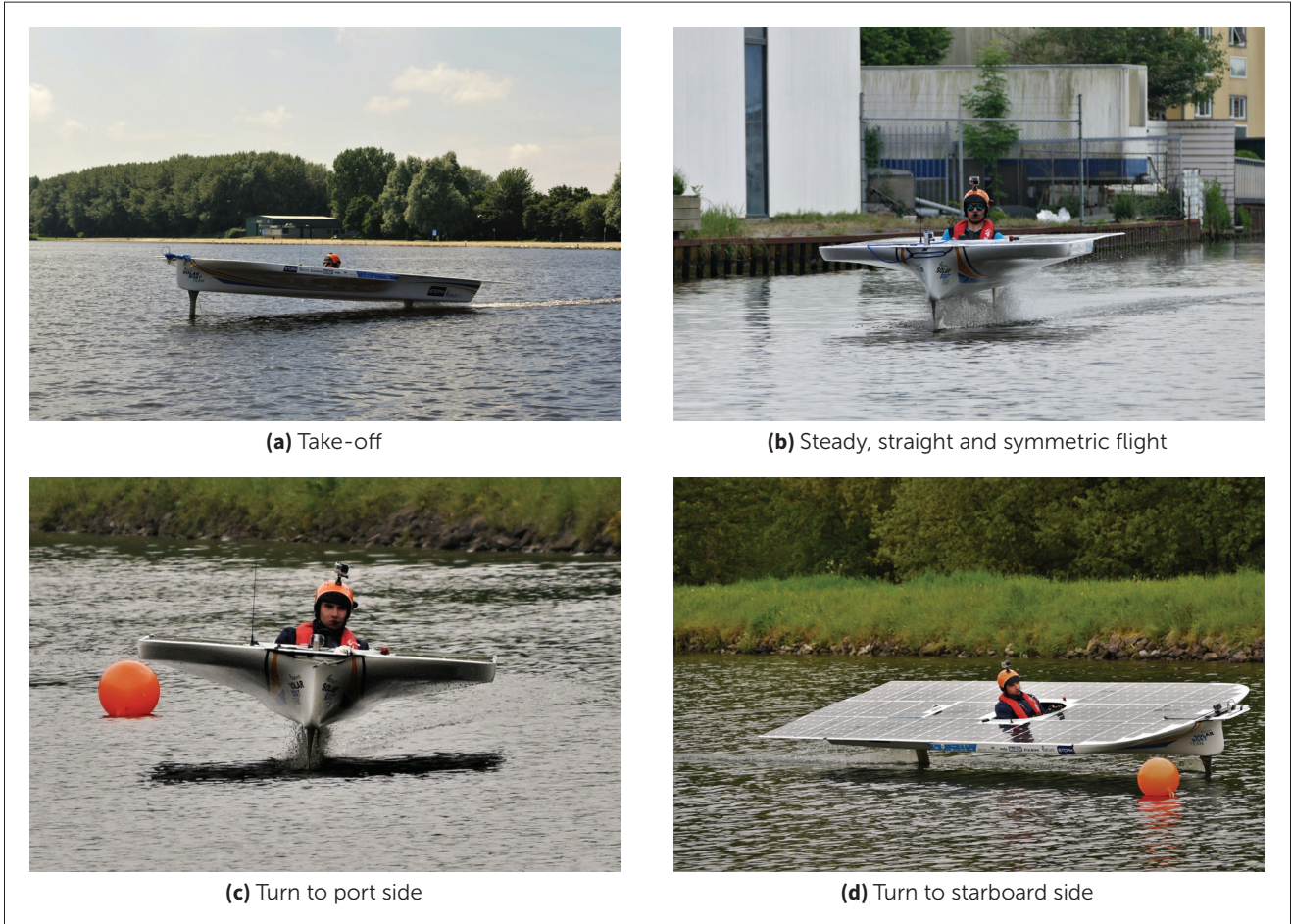
FIGURE 3. Four typical maneuvers of a single-track hydrofoil boat: the TU Delft Solar Boat 2016.
