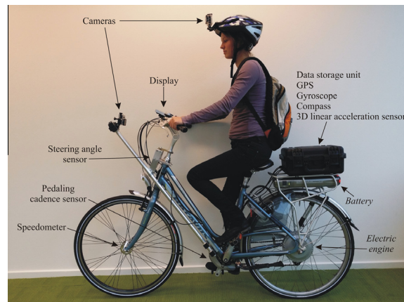
Fig. 1. The instrumentation of the pedelec. The instrumented conventional bicycle was not fitted with the battery and electric engine (indicated in italics).
