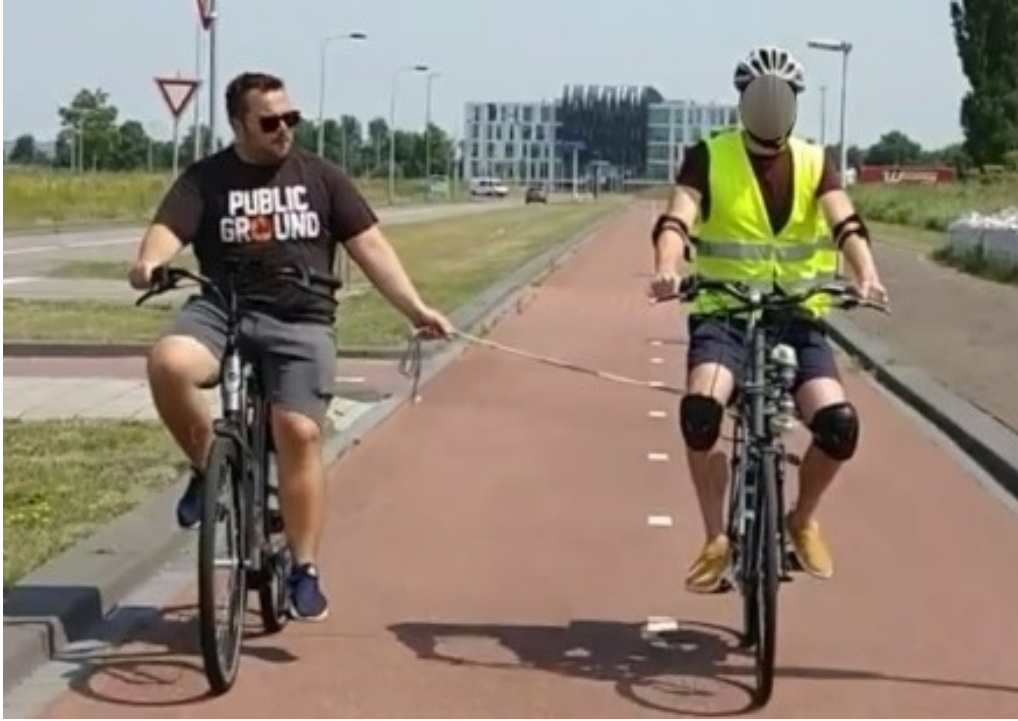
Figure 2: Experimental trial performed across Heertjeslaan cycling path of TU Delft; Experiment coordinator cycling next to steer-by-wire bicycle while pulling laterally the subject with a rope.
