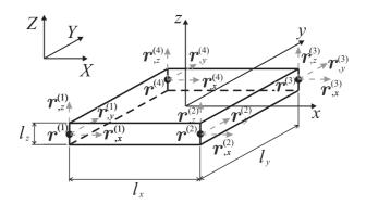
Figure 1: Undeformed plate element with its dimensions in current configuration.
