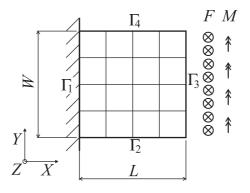
Figure 2: Loading, boundaries and uniform  $4 \times 4$  mesh of a square cantilevered plate with quadrilateral elements.
