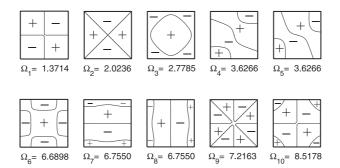
Figure 4: First 10 transverse vibration modes together with their dimensionless frequencies for free (ffff) square plate as calculated by the ANCF-P48lsa with a mesh 32 x 32 and Poisson factor  $\nu$ =0.3. A relative plate thickness of H/L =0.01 was used.
