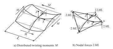
Figure 5: Particular cases of pure bending caused by distributed twisting moment M and nodal forces 2ML.
