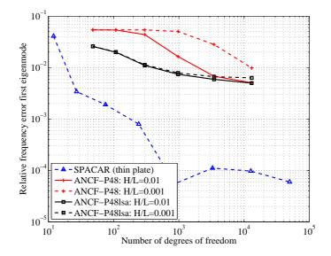
Figure 3: Convergences of the first mode normalized by analytical solution for free (ffff) square plate as calculated by the SPACAR, ANCF-P48 and ANCF-P48Isa with Poisson factor  $\nu$ =0.3.Two different relative plate thickness of H/L=0.01 and H/L=0.001 were used.
