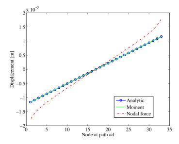
Figure 7: Displacements at asymptotic line ad, mesh  $64 \times 64$ , ANCF-P48lsa, H/L = 0.2.
