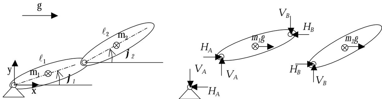
**Figure 1** Double pendulum and free body diagrams.
