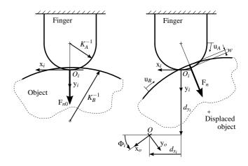
Figure 2. Local surface frame and orthogonal frame at a contact point, adapted from [1].
