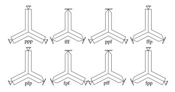
Figure 4. Limit cases of zero and infinite contact curvatures. Letter p denotes *pointed* finger, f denotes *flat* finger tip, and the  $i^{th}$  letter belongs to the  $i^{th}$  finger.
