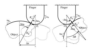
Figure 3. Relative motion of the object by slip (left) and roll (right).
