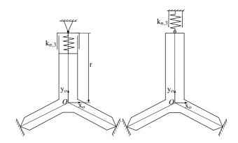
Figure 5. Grasp with finite stiffness at contact 3 in the object (left) and in the finger (right), respectively.
