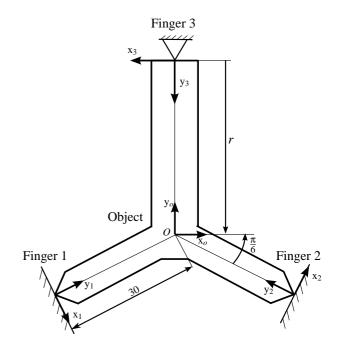
Figure 1. Grasp of a polygon by rigid fingers with zero (Finger 1 and 2) and infinite (Finger 3) curvature, adapted from [1]. Dimensions in [mm], [rad].
