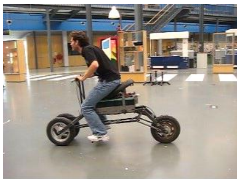
figure 2: left: instantaneous pole position of the mechanism, right: the test-rig to test the tilting on the perceived comfort.
