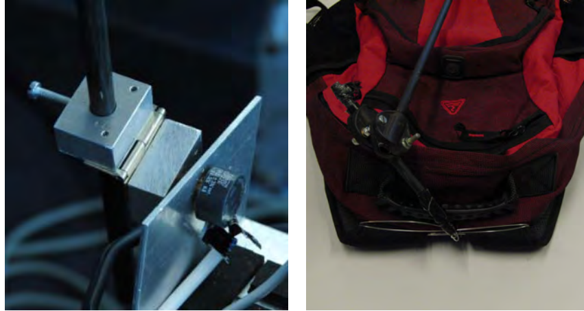
(a) The potentiometer which is used in order to measure the body movement of the rider, the arm that is also connected to the backpack is also shown. (b) The arm connected to the backpack. The arm is connected to the backpack as rigidly as possible using iron wire. Figure 5.1 shows an overview of this system.
