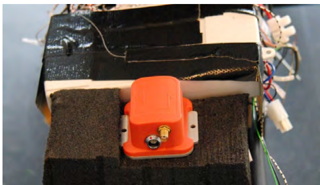
Figure 5.7: The Xsens MTI-g orientation sensor on the location where it was connected to the measurement bicycle. The sensor was fixed rigidly to bicycle frame using duct tape with the foam material from the picture between the frame and the sensor. The purpose of the foam material is to provide some damping for the vibrations caused by the road’s surface.
