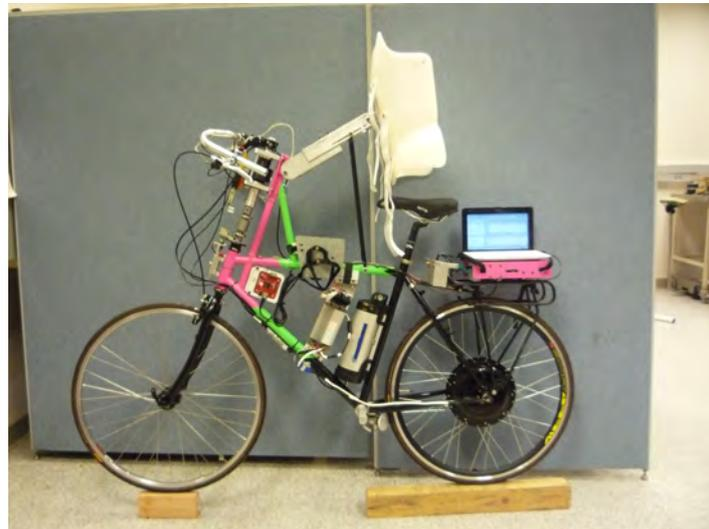
**Figure 3-1:** Photo of the measurement bicycle which is used for rider identification in bicycling. Source: [picasaweb.google.com/moorepants](https://picasaweb.google.com/moorepants).
