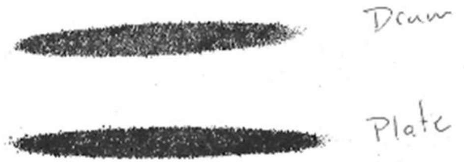
Figure 3-2: Ink prints of contact patches of a Maxxis radial.
