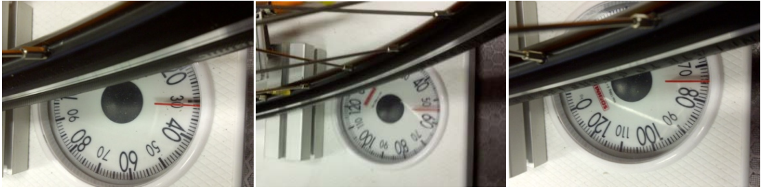
Figure 3-21: Vertical load created by attaching additional masses to frame of test device number 3.
