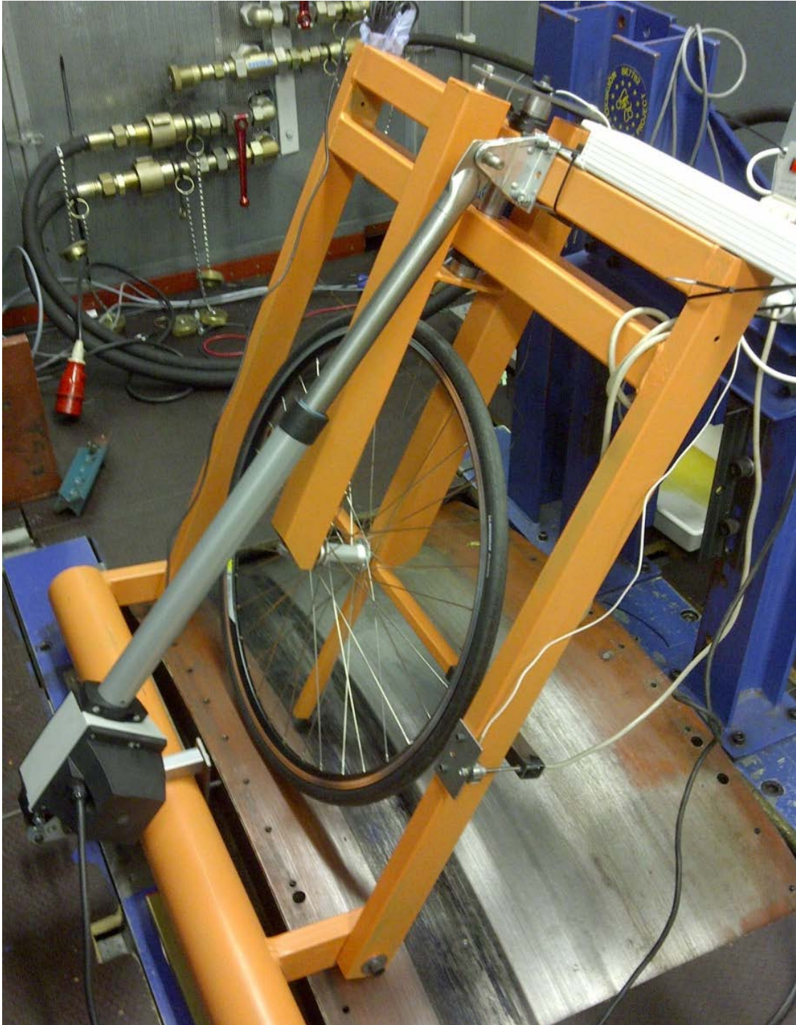
Figure 3-19: Camber angle actuator installed on test device number 3 before non-skid tape is installed on the drum.
