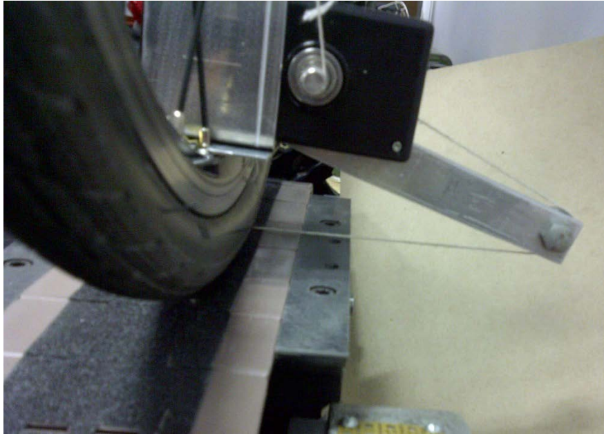
Figure 3-14: Measuring tire centerline lateral deflection beyond the contact patch.
