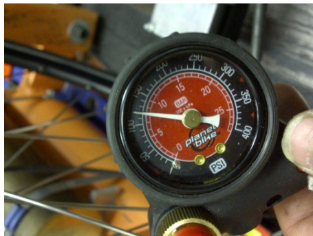
Figure 3-22: Inflation pressure gauge integrated with tire pump.
