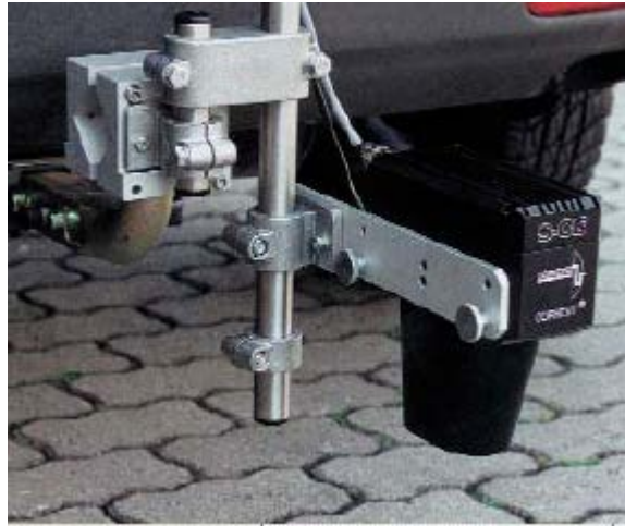
Figure 3-34: Contact-less optical sensor for measuring sideslip angle.
