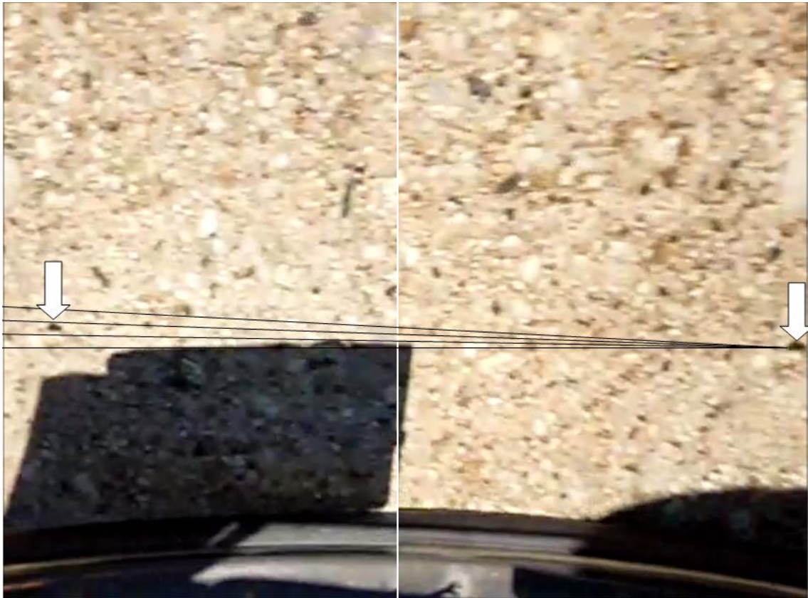
Figure 3-33: Extracting slip angle from sequential video frames.
