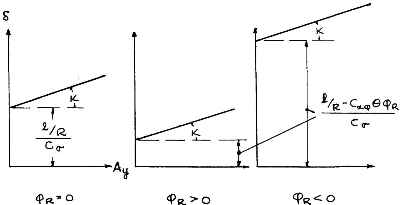
In other words a constant radius skid-pad test should reveal the understeer factor,  $K$ , regardless of rider lean angle - a result which is encouraging since we had earlier suspected that lean might "contaminate" the results.
