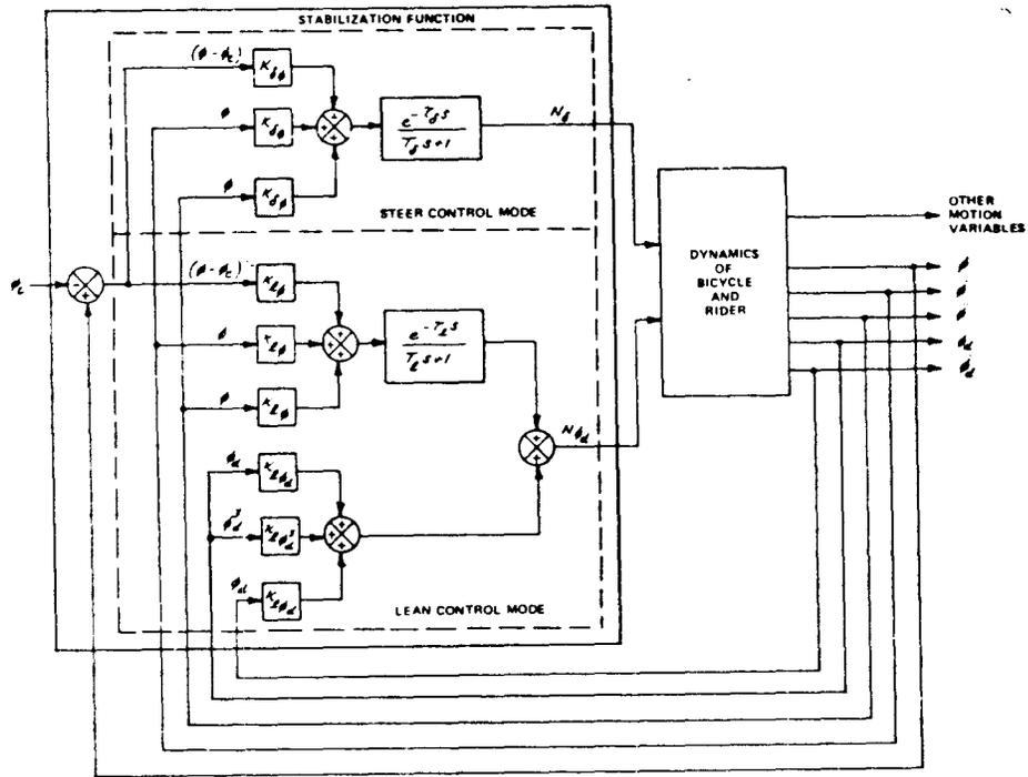
Block Diagram of Stabilization Function of Rider Control Model
