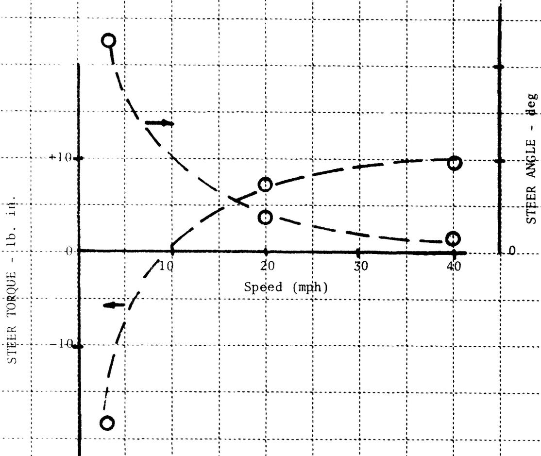
FIGURE 20: DIRECTIONAL CONTROL RESPONSE CHARACTERISTICS - ON-CENTER PERFORMANCE (HONDA 360)
