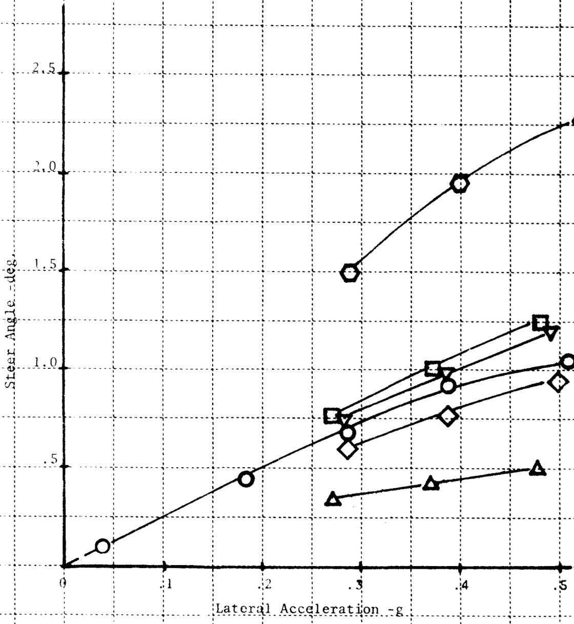
FIGURE 16: SIMULATED DIRECTIONAL CONTROL RESPONSE CHARACTERISTICS - STEER ANGLE
