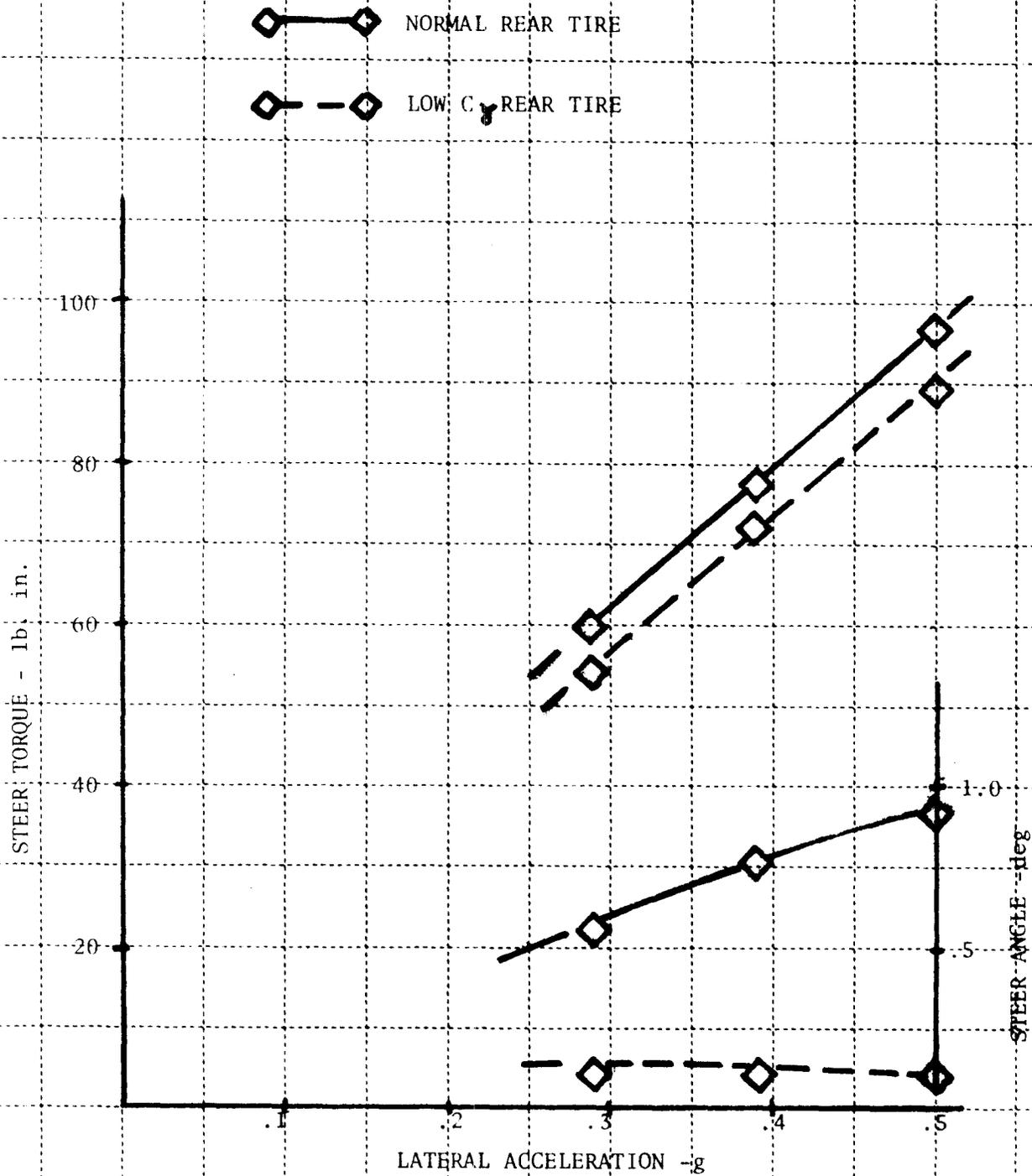
FIGURE 23: DIRECTIONAL CONTROL RESPONSE CHARACTERISTICS - TIRE EFFECTS ON YAMAHA
