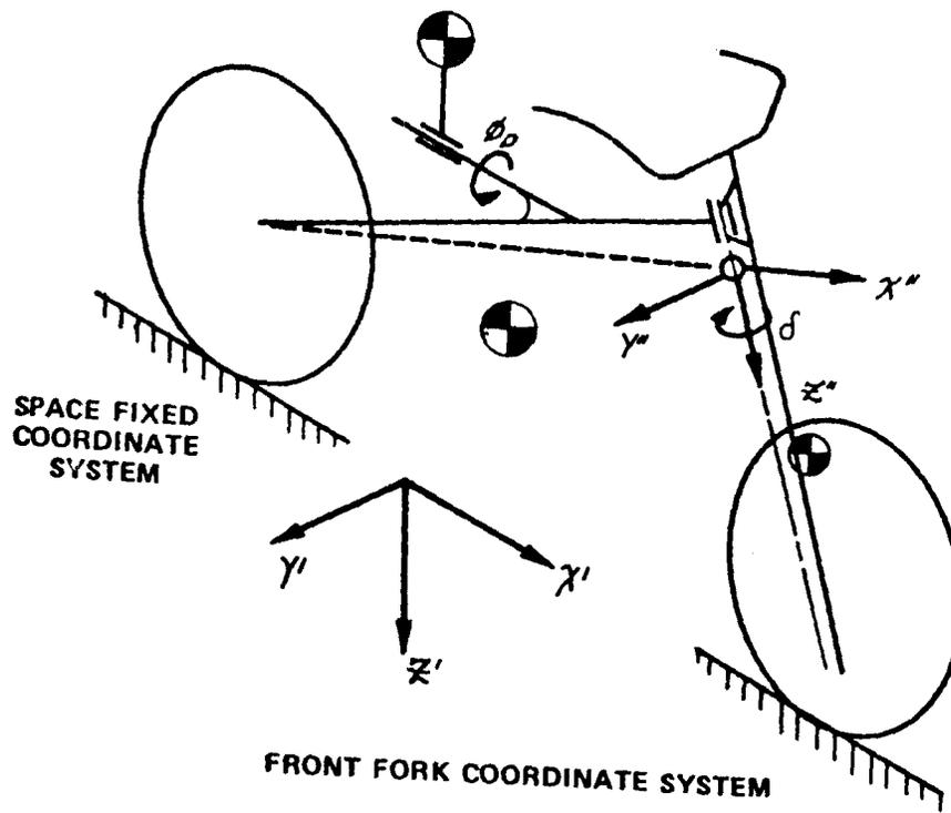
Figure 10. Two-Wheel Vehicle Model
