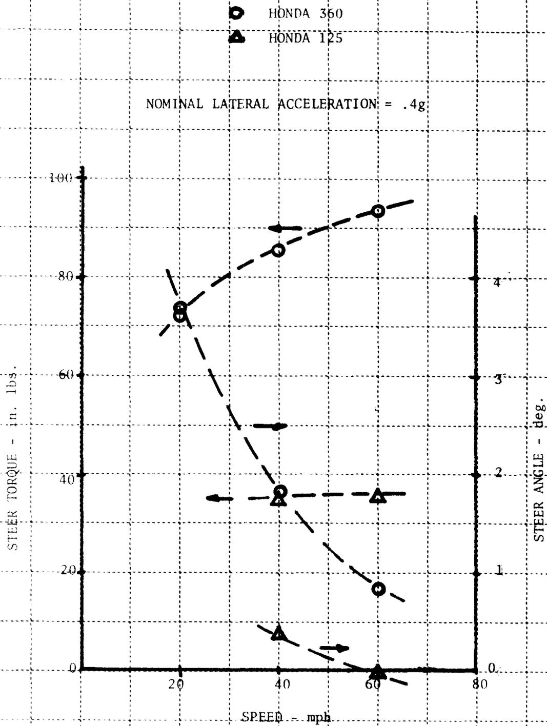
FIGURE 18: DIRECTIONAL CONTROL RESPONSE CHARACTERISTICS - SPEED EFFECTS
