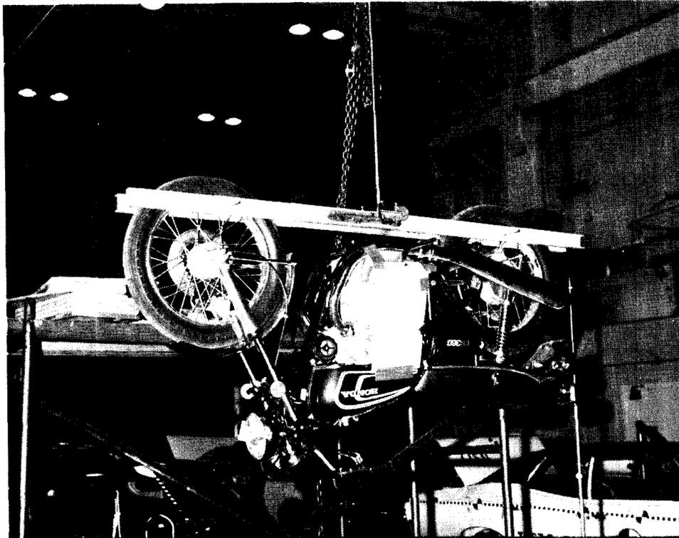
Figure 1a MEASUREMENT OF YAW MOMENT OF INERTIA ( $I_{ZZ}$ )
