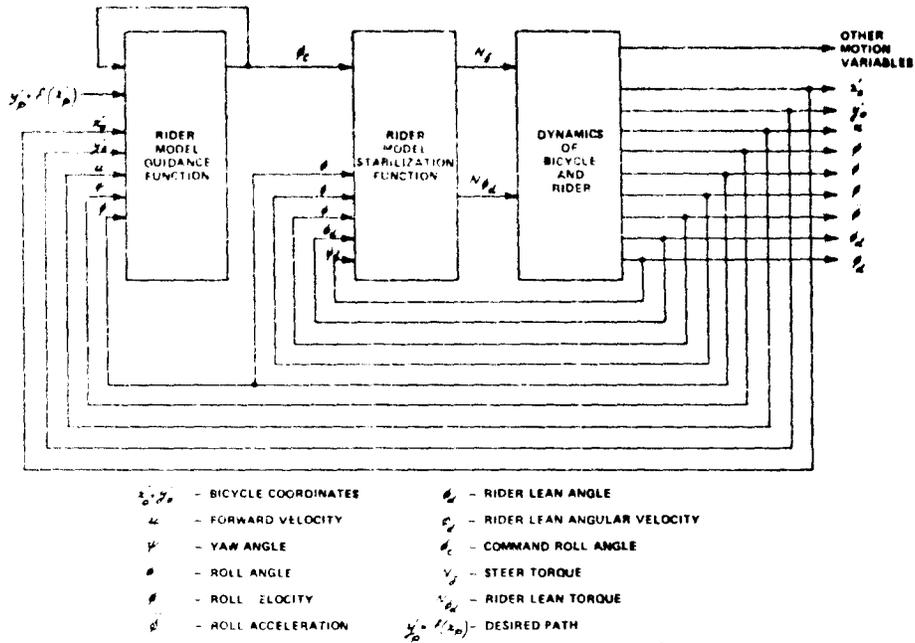
Fig. 12. Block Diagram of Rider Control Model
