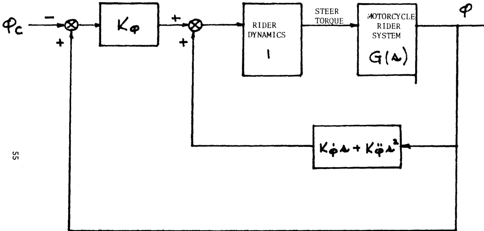
FIGURE 14: MOTORCYCLE STABILIZATION LOOP
