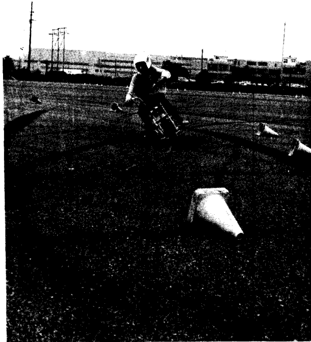
Figure 14 HARD CORNERING IN THE MINIBIKE LATERAL ACCELERATION TEST [Note foot peg on inside]
