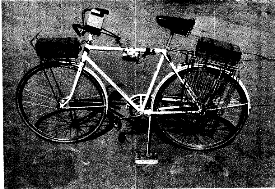
Figure 4.1 STANDARD BICYCLE WITH 12½ POUND LOAD ON BOTH FRONT AND REAR CARRIERS
