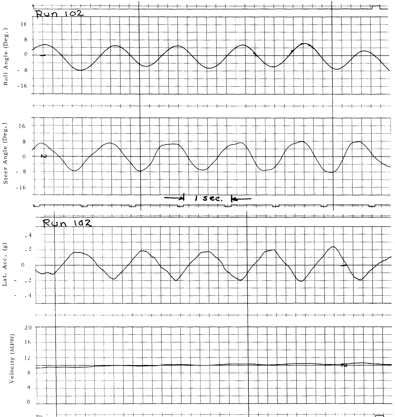
Figure II.3 Run 102, Narrow Slalom Course - Low Front Tire Pressure
