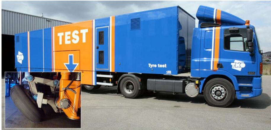
Figure 5. TNO Tyre Test Trailer and test tower for motorcycle tyres.
