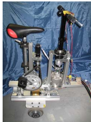
Figure 21. Prototype vehicle of the two-wheeled inverted pendulum vehicle moved by human pedaling
