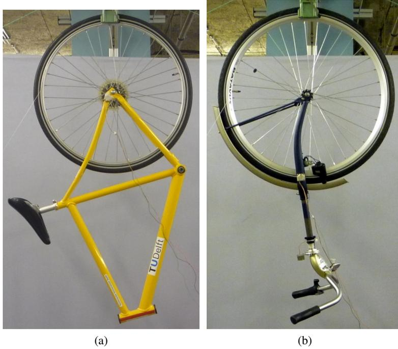
Figure 11: (a) Rear frame hung as a compound pendulum. (b) Browser fork hung as a compound pendulum.
