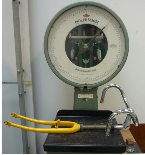
Figure 3: The scale used to measure the mass of each bicycle component.
