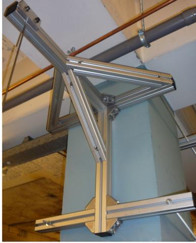
Figure 8: The rigid pendulum fixture mounted to a concrete column.
