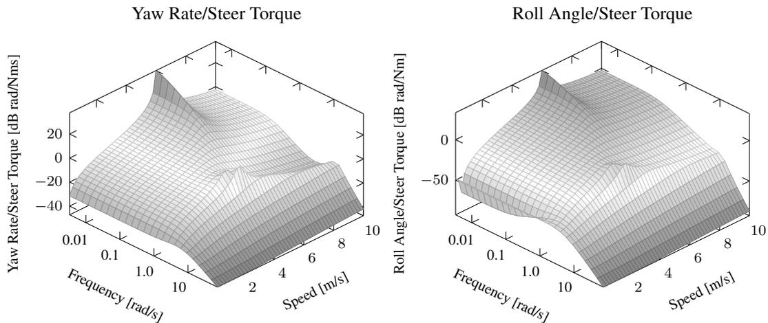
**Figure 2.** Speed Dependent Bode Plots of Bicycle
