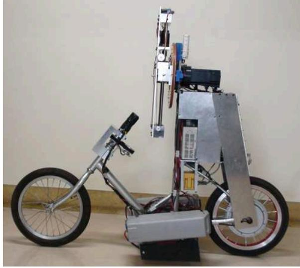
**Figure 3.** Bicycle with flywheel balancer hardware.
