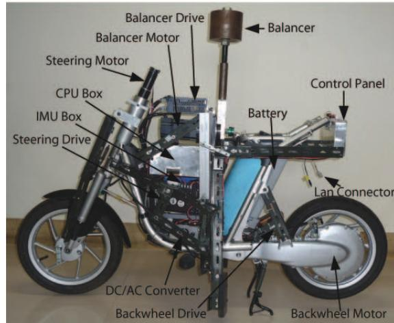
**Figure 1.** Bicycle with a balancer system.
