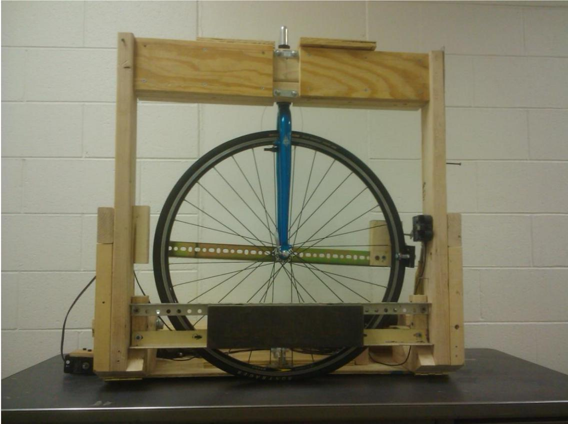
**Figure 5.** The test device showing the wheel held in place with a bicycle fork and the turnbuckles used to alter its orientation. Two for camber angle, and one for steer angle.
