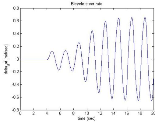
**Figure 10** Bicycle steer rate versus time at an unstable weave velocity  $v=4.0$  [m/s].
