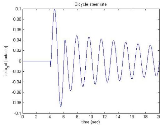
**Figure 12** Bicycle steer rate versus time at a stable weave velocity  $v=4.5$  [m/s].
