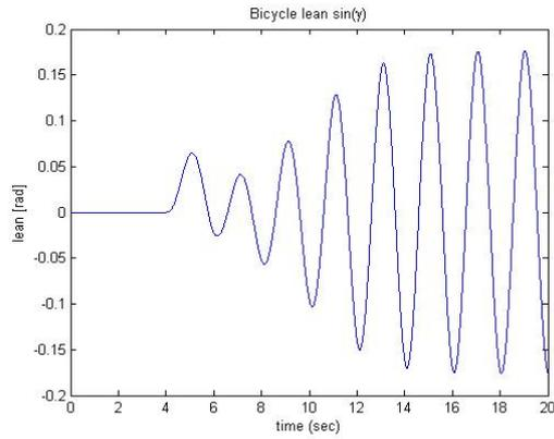
**Figure 9** Bicycle lean versus time at an unstable weave velocity  $v=4.0$  [m/s].
