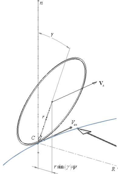
**Figure 2** The wheel disc under camber angle  $\gamma$ , illustration of the difference between the path of  $c$  and of the wheel centre  $a$
