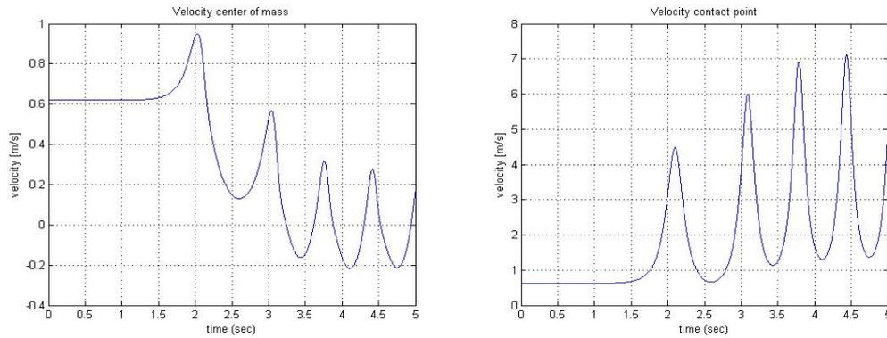
**Figure 4** Velocity as a function of time. Simulated with a initial forward velocity of 0.62 [m/s] centre of mass  $a$  and contact point  $c$  respectively.
