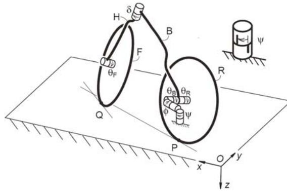
**Figure 6:** The ‘Whipple’ or benchmark bicycle, picture taken from [2]
