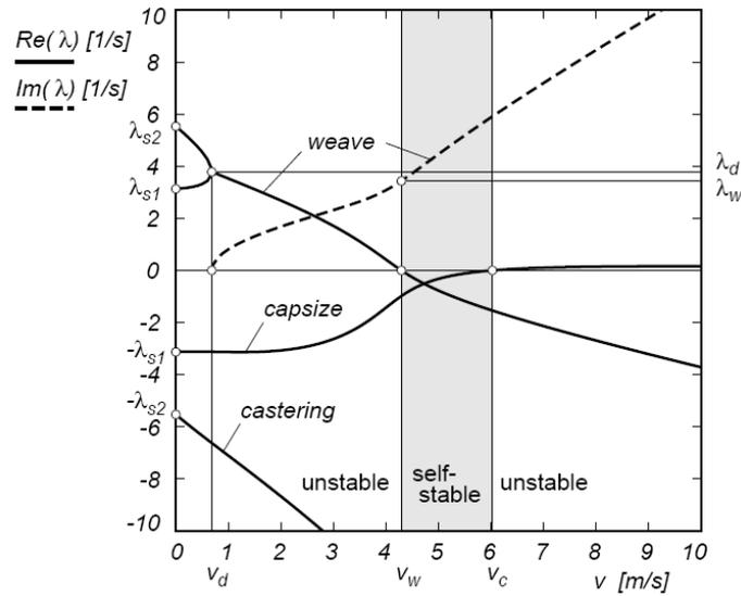
**Figure 7:** Eigenvalues  $\lambda$  from the linearized stability analysis for the benchmark bicycle. The solid lines correspond to the real part of the eigenvalues and the dashed line corresponds to the imaginary part of the eigenvalues, in the forward speed range of  $0 \leq v \leq 10$  m/s. graph taken from [2]
