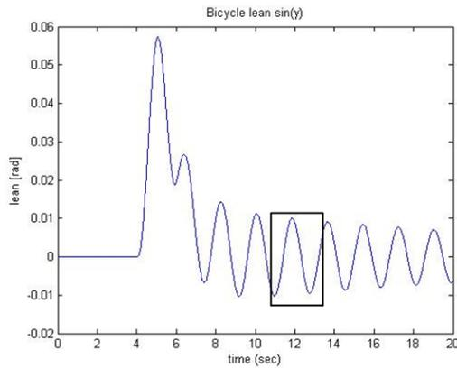
**Figure 11** Bicycle lean versus time at a stable weave velocity  $v=4.5$  [m/s].
