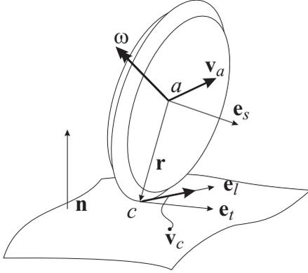
**Figure 1.** The wheel disc with contact point location  $r$
