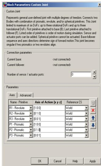
**Figure 5** The SimMechanics graphical interface (GUI) that allows custom degrees of freedom to be assigned to the body
