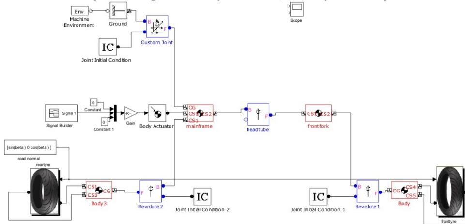
**Figure 8** Overview of the SimMechanics model structure with its four bodies as red blocks, the interconnecting revolute joints presented as blue blocks, and a dedicated front and rear wheel module.
