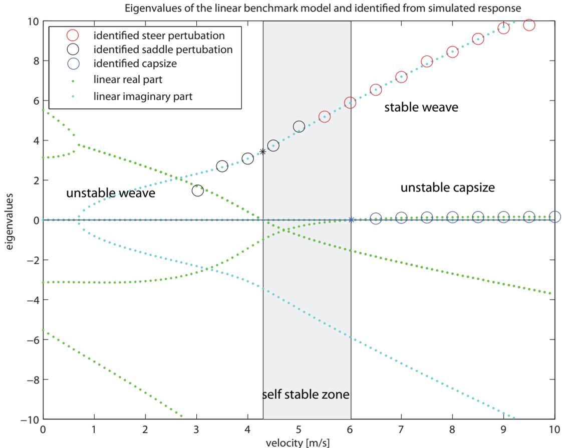
**Figure 13** The eigenvalue versus speed for both benchmark bicycle and the SimMechanics
