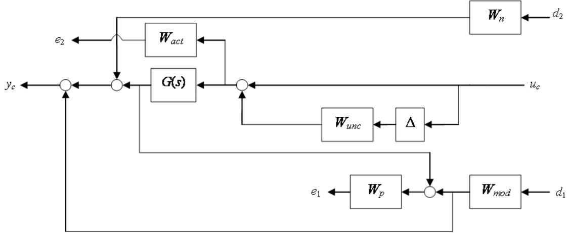
Figure 5. General structure of the system, for the design of the  $\mathcal{H}_\infty$  controller.
