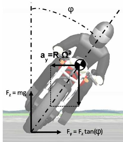
**Figure 9.** Steady turning: roll angle and lateral acceleration of the motorcycle equipped with zero thickness tires.
