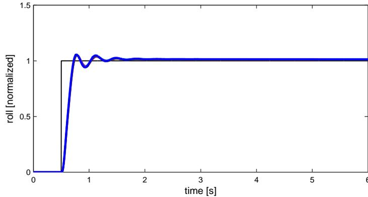
**Figure 8.** Closed-loop step responses of the LPV controlled system for several different longitudinal velocities and lateral accelerations.
