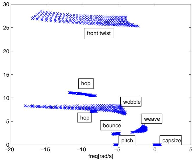
**Figure 3.** Vibrational modes for different longitudinal velocities and lateral accelerations.
