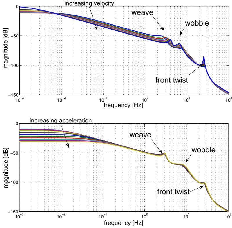
**Figure 4.** Bode diagrams of the linearized models. Upper plot: constant lateral acceleration  $a_y = 0 \text{ m/s}^2$ , velocity  $v = [25, 60] \text{ m/s}$ ; Lower plot: constant velocity  $v = 30 \text{ m/s}$  velocity  $a_y = [0, 12] \text{ m/s}^2$ .
