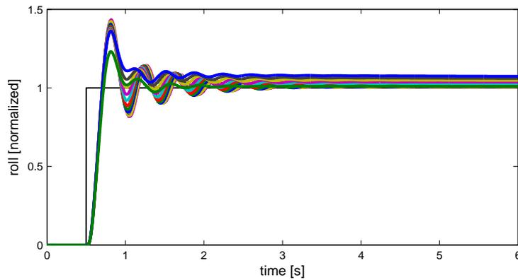
**Figure 7.** Closed-loop step responses for several longitudinal velocities and lateral accelerations.
