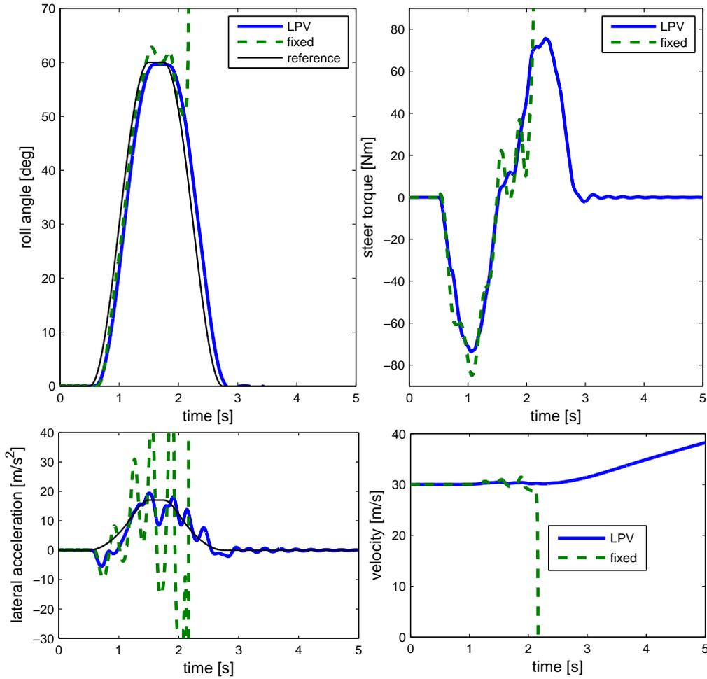
**Figure 11.** Comparison between the  $\mathcal{H}_\infty$  controller and the LPV controller for an aggressive cornering maneuver: roll angle, steering torque, lateral acceleration and longitudinal velocity.
