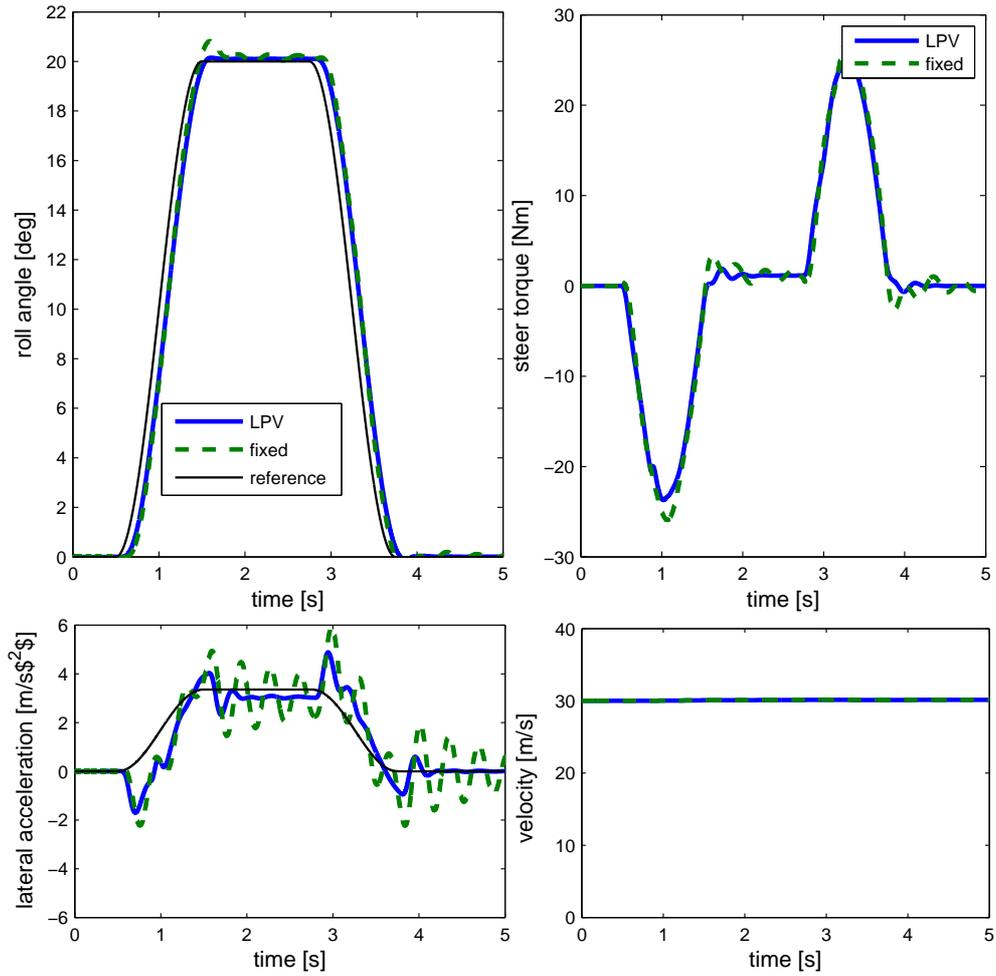
**Figure 10.** Comparison between the  $\mathcal{H}_\infty$  controller and the LPV controller for a gentle maneuver: roll angle, steering torque, lateral acceleration and longitudinal velocity.
