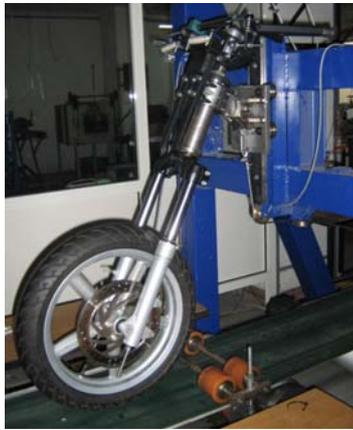
Figure 1 - Castor on belt rig
