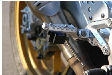
Figure 3. A laser sensor for lean-angle estimation.
